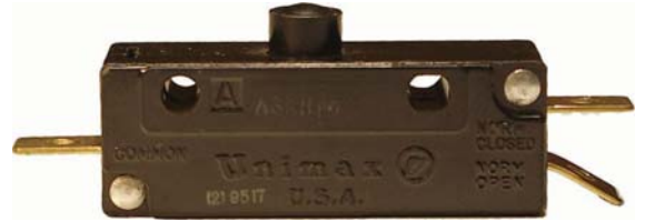
SW-37 SPDT MOM. ON AND/OR MOM. OFF 20 amp. 125 & 250 VAC
