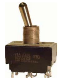
7563K4 DPDT ON - OFF - ON 7565K5 DPDT ON - ON 15 amp. 125 volt
